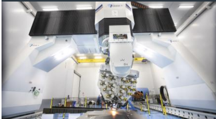
Automated Fiber Placement: Automated manufacturing
