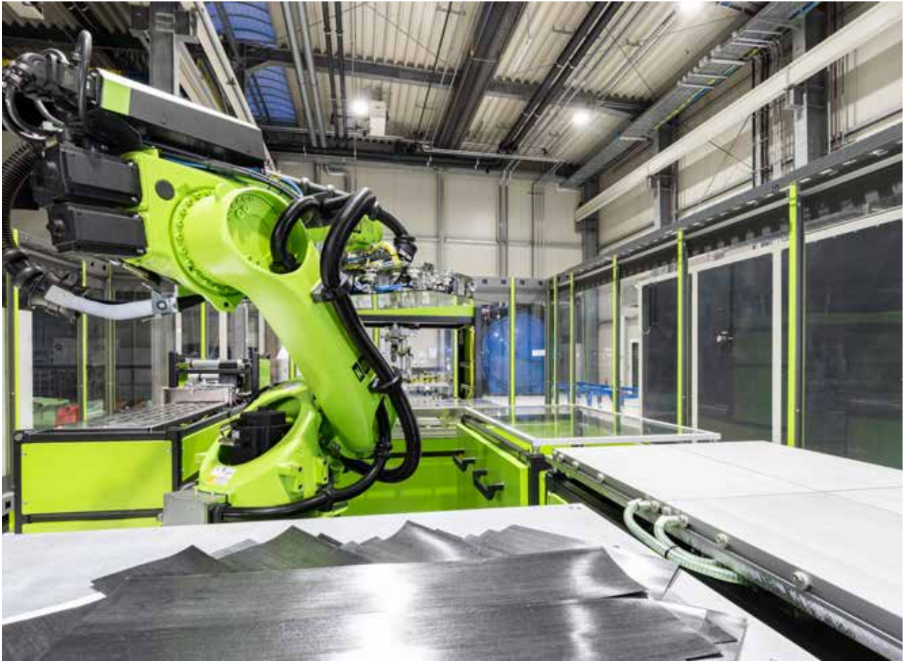
ENGEL pick & place fiber placement system for thermoplastic fiber-reinforced composites
