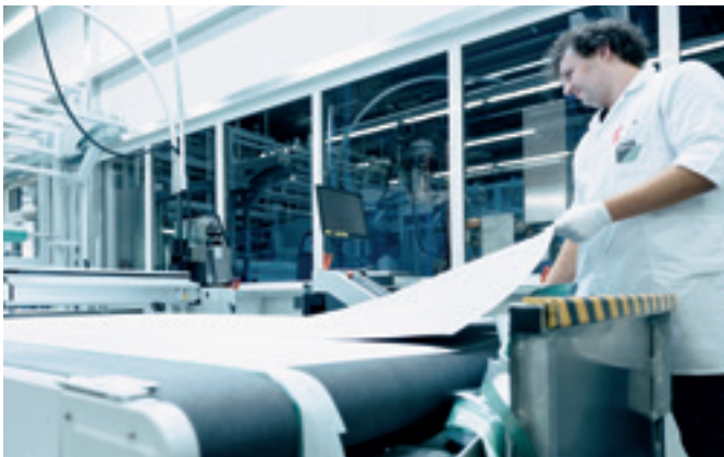
Prior to further processing, carbon fibre sheets undergo high-precision cutting operations.
