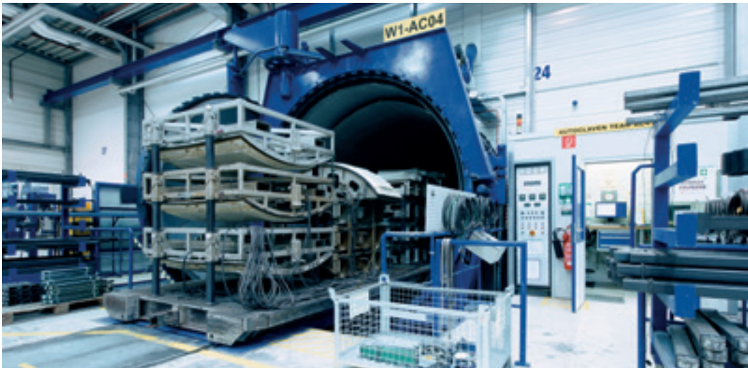
Composite parts’ curing process in the autoclave
