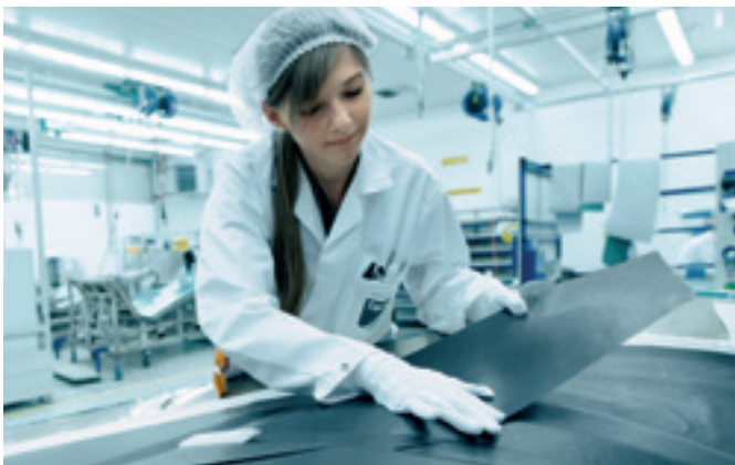
In a clean room the carbon fibre outer skin is applied manually.
