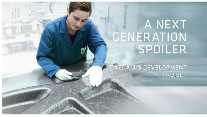
A development engineer at FACC laying out by hand the layered woven carbon fibre mats to create the backbone for the prototype.
