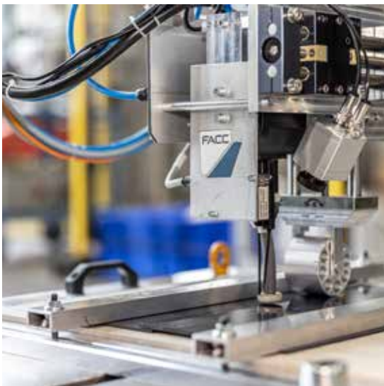
Induction welding head for joining thermoplastic components
