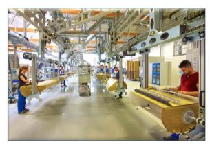
Interior: A320 Moving Line with 18% efficiency increase
