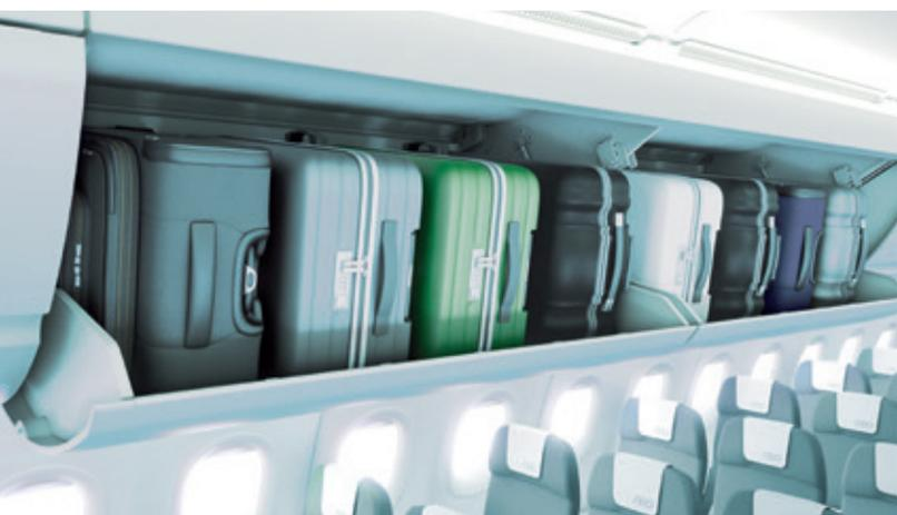
*FACC's new movable bins provide ten percent more stowage volume and facilitate loading and unloading.*
