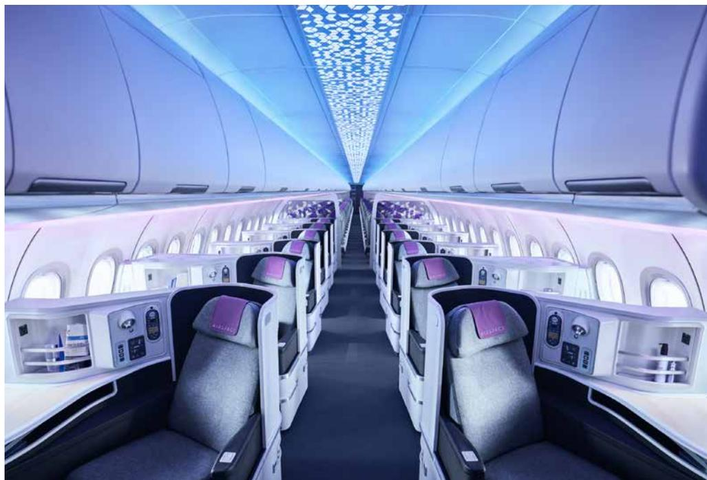
The Airspace cabin, which FACC developed for the Airbus A320 and has been producing since 2021, makes an important contribution to consistent weight optimization and thus to lower fuel consumption through the use of innovative fiber composite materials and novel manufacturing technologies.
