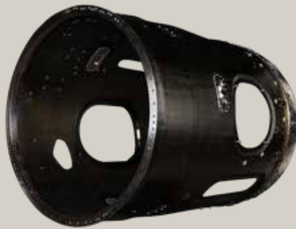
OUTER BYPASS DUCT
